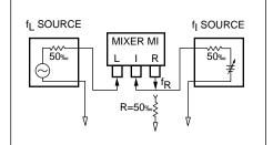
The amount of signal passing through the mixer from the L-port to the R-port is determined by the dc control current present at the I-port. Maximum attenuation is
