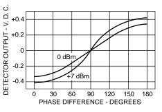
Typical Phase Detector Output vs. Phase Difference
