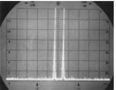
High drive: With a +27 dBm fL drive level, a high power mixer virtually eliminates all two-lone products from the 60 dB spectrum.
