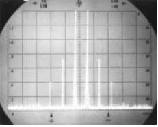
Medium drive: With a +17 dBm fL drive level, a higherpower mixer provides an additional 12 dB of suppression of the third-order product.
