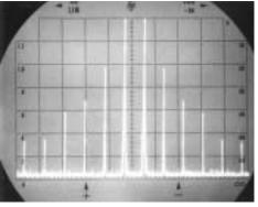
Low drive: With a +7 dBm fL drive level, a balanced mixer can suppresses many of the two-tone spurs. However, a number of relatively unsuppressed products remain
