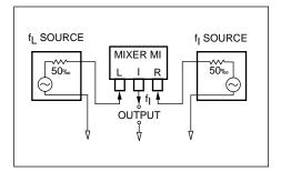
A balanced mixer may be used for phase detection. With identical frequencies connected to the R- and L-ports, a dc output related to the phase difference between the
