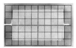
For pulse modulation, feed the unmodulated signal to the L-port and the modulating pulse to the I-port. No dc offset current should be used. Pulse lengths can be of unlimited length since the I-port is direct coupled. A 20 mA level is sufficient to fully turn on the diodes. Rise and fall times less than 1 nsec can be achieved. Zero current turns the diodes off. Either a positive or a negative pulse may be used.
